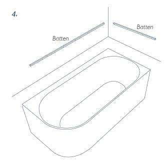
Due to the design and production methods of the Flow Bath there will be a small gap between the top ledge of the Bath and the wall, we recommend that the bath is fitted up to the bare wall and the tiling works should finish at the top ledge of the bath, The seal can be completed with a continuous bead of silicone sealant to complete the watertight seal required.
