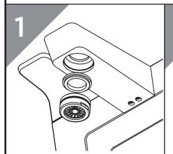
Loosen aerator using a spanner, Remove the aerator and the washer
