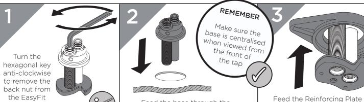
Feed the base through the sink hole from the top.
