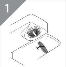
Loosen flow straightener using a coin.
