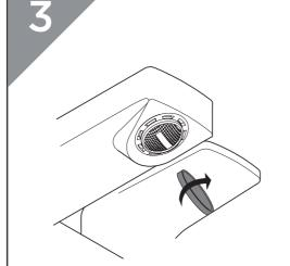
Replace the flow straightener, ensuring the washer has been fitted. Tighten in place by using a coin.
