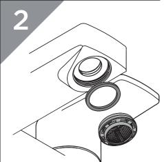
Remove the flow straightener and the washer.
