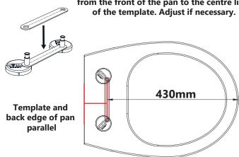
Once the template is in place and correctly positioned (430mm +/- 3 from the front of the pan to centre line of the template), hold the hinges securely and tighten the fixing screws with a screw driver. Remove the template.
