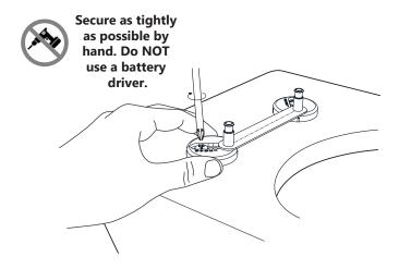
Amenasure the distance, making sure the 430mm dimension is met and remove the template and add the cover cap.
