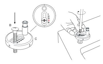
Using the anchor template provided, place over the two pins, making sure the template is parallel to the back of the pan and the pins are facing toward the bowl.
