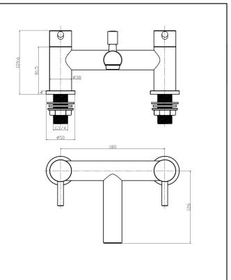
Dimensions (measurements in mm)
