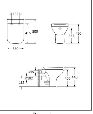
Dimensions (measurements in mm)
