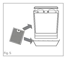
it with hot soapy water. You can also wash the grease filter in a dishwasher, ensuring that you place it in an upright position to prevent damage from other items in the dishwasher.
