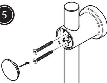
Fit the top bracket to the rail and secure in place using the fixings supplied. Fit the end caps to both brackets.
