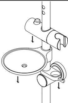
Fit the hose retainer, shelf and slider to the rail.
