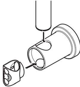
Insert the clamp and slide the rail through the bottom bracket.
