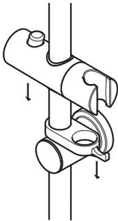
Fit the hose retainer and slider to the rail.
