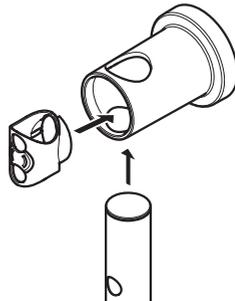
Insert the clamp and slide the rail through the top bracket.
