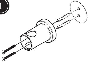
Mark the position of both wall brackets bearing in mind the height of different users. Secure the bottom bracket to the wall using fixings supplied.
