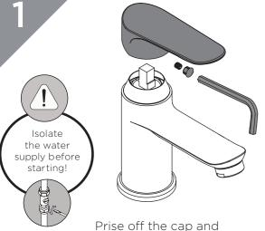
Prise off the cap and undo the grub screw to remove the handle.
