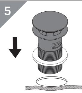
Feed the waste body through the basin, ensuring the rubber washer is in place.
