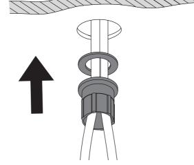
Connect the flexible tails to the hot and cold water supplies.
