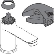
Unscrew the shroud. Undo the cartridge retaining nut to remove the cartridge.
