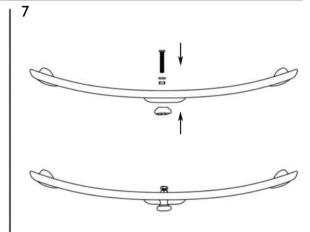
Attach the Ashpan Handle to the Ashpan using Ix M6 Bolt, Ix M6 Washer and Ix M6 Nut.
