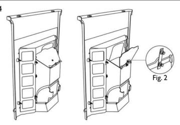
Solid Fuel Usage: Rest the Damper Plate onto the grove on the back of the Fireplace Fascia.
