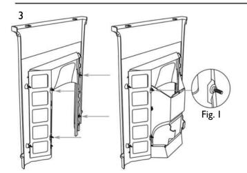
Insert the 4 M6 Studs into the back of the Fireplace Fascia. Attach Fireplace Back to the back of the Fireplace Fascia, ensuring that the M6 Studs pass through the fixing brackets on the Fireplace Back. Secure and tighten using 4 M6 Washers and 4 M6 Nuts.
