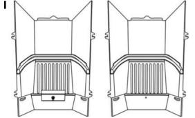
Remove the Firebrick Retaining Plate by removing the 1 x M6 Stud, Washer and Bolt.
