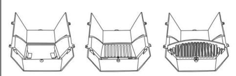
Lay Fireplace Back down on level ground. Position Firebrick in place and then insert I  $\times$  M6 Stud into the hole just below the Firebrick. Insert Grate into the groves on the Fireplace Back, passing the fixing lug over the M6 Stud. Secure in place with I  $\times$  M6 Washer and I  $\times$  M6 Bolt.
