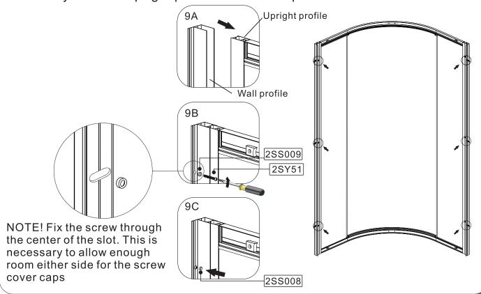
After your wall profiles have been fixed you can square your enclosure on the tray and fix the wall profiles to the upright profiles as shown below. 10A.From inside drill the frame top, middle and bottom making sure to step in a Min. 14mm from the edge of the frame.
