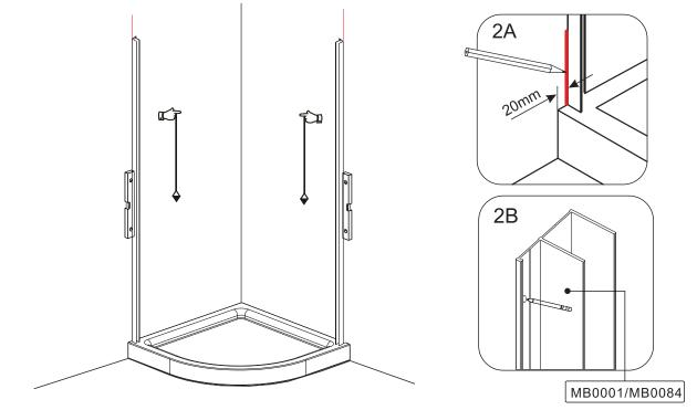
Remove the wall profiles and use a 6mm masonary drill bit to drill the holes for your fixings and place the wall plug into the holes.
