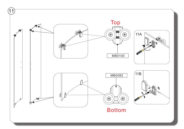
To fit your door panels first hang the top roller to support the weight of the glass panel. Push down the bottom roller fully and guide the roller into the bottom track.
