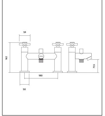
Dimensions (measurements in mm)
