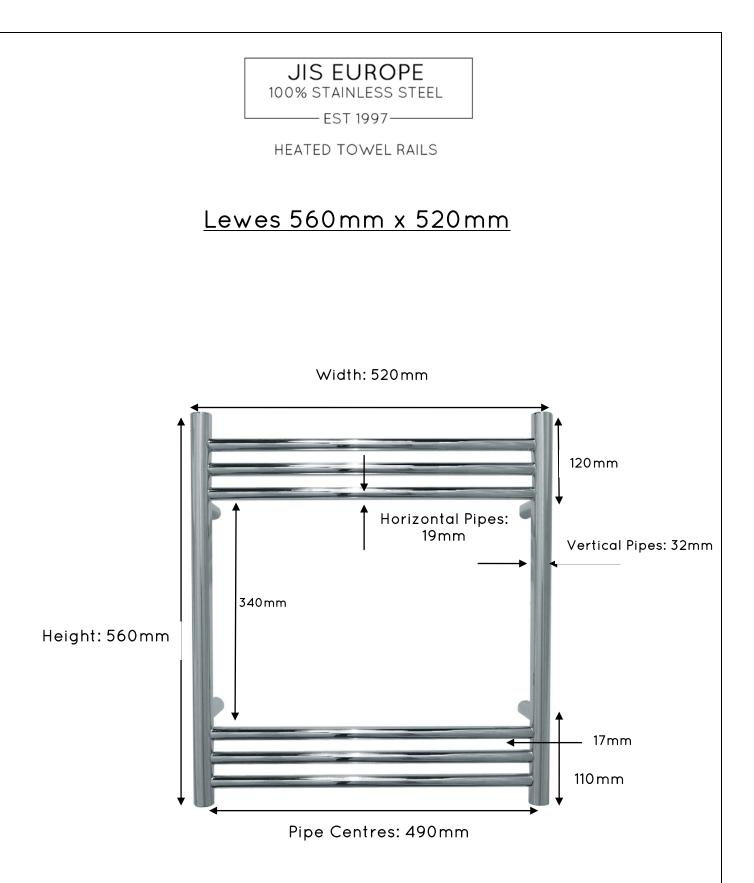
Overall Projection: 117mm\* Pipe Centres from the Wall: 102mm \*When using short brackets, projection and pipe centres from wall will be reduced by 25mm.
