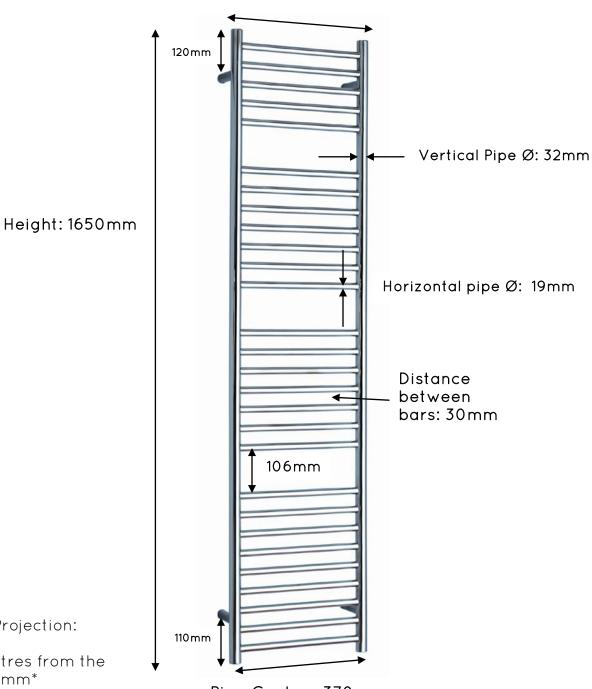
Overall Projection: 117mm\* Pipe Centres from the Wall: 102mm\*
