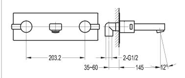
Dimensions are in millimetres except thread sizes which are BSP imperial.
