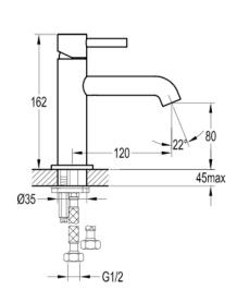
Dimensions are in millimetres except thread sizes which are BSP imperial.
