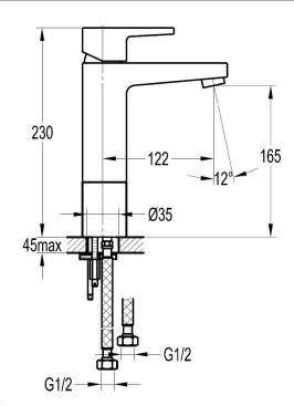
Dimensions are in millimetres except thread sizes which are BSP imperial.
