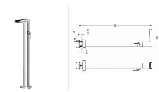
Dimensions are in millimetres except thread sizes which are BSP imperial.
