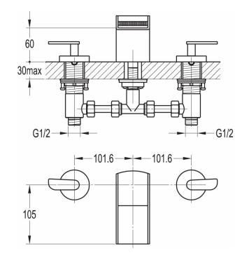
Dimensions are in millimetres except thread sizes which are BSP imperial.
