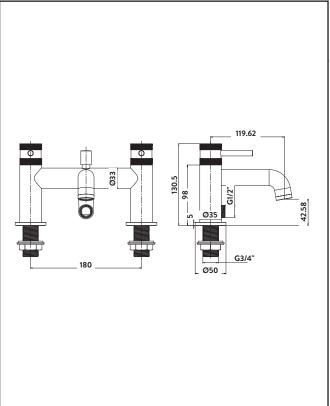
Dimensions (measurements in mm)
