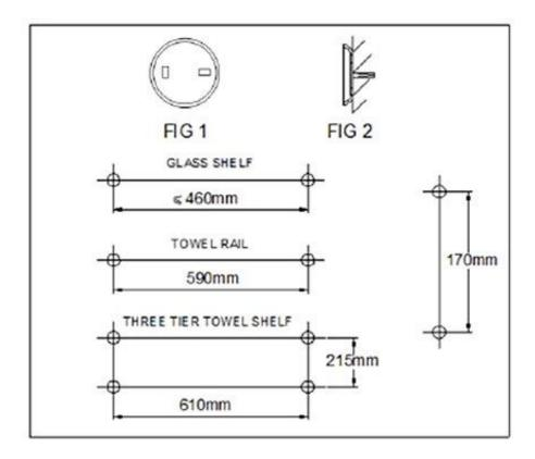
**NOTE:** All dimensions refer to the pillar centers. Guide dimensions only, all centres should be measured & checked prior to drilling.
