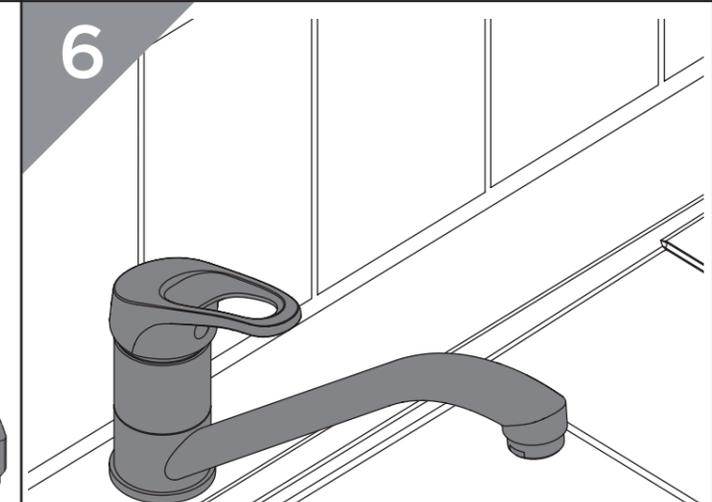
Turn on the water supply. Check all joints and connections for any leaks.
