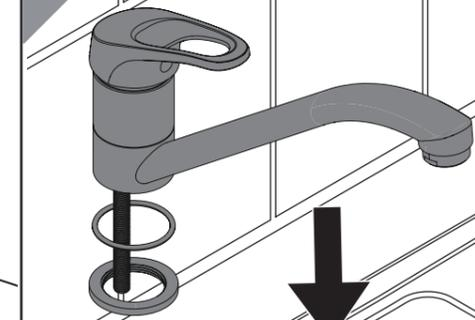
Feed the tap body through the tap hole, ensuring the plinth and washer are in place.
