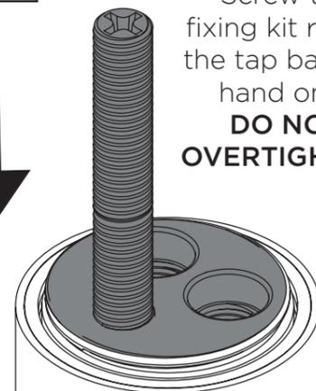
Screw the fixing kit rod to the tap base by hand only. **DO NOT OVERTIGHTEN.**
