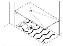
(3) Add adhesive to the wooden base (or wedi type board) base applied in 10mm strips with a distance of 50mm between them and fix the tray to the base checking that it is perfectly level (4 sides checking).
