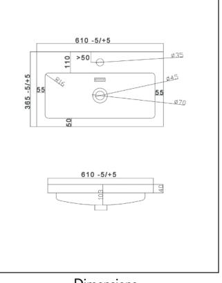
Dimensions (measurements in mm)
