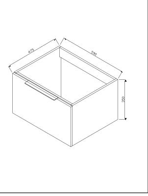
Dimensions (measurements in mm)
