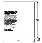
Adittional notes: Important: Please check cut out details carefully before cutting worktops, size shown is flush to bowl edge Overall product size: 380 x 438 x 205 corner radius 10mm
