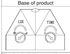
Duration the bulb stays on is adjustable by turning 'TIME' screw
