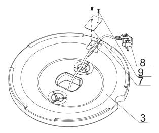
Fasten the power cable with the cord clip (7) and fix it to the base (3) with the screws (9).
