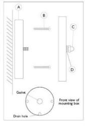
Having correctly identified the wiring from your existing light fitting, pull the wire through the hole and connect to the connection block inside the product in the following
