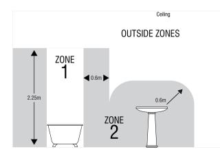
This product is suitable for use in Zone 2 and outside Zones of a bathroom. See diagram. If this unit is being fitted in a room containing a bath or shower, a 30mA RCD must be used, in accordance with IEE regulations.
